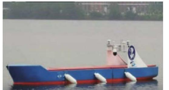
Fig. 6 KVLCC2 under-actuated model ship
